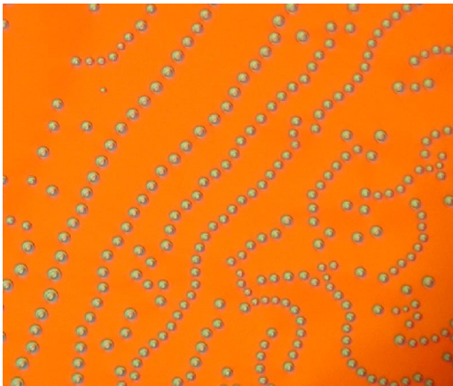
FIG. 1. (Color online) Chains of isotropic droplets in a smectic film (approximately 300-nm film thickness) of the material 11OAB, observed in unpolarized white light near the clearing point, droplet diameters in the range of 2–5 \mu\text{m} .
